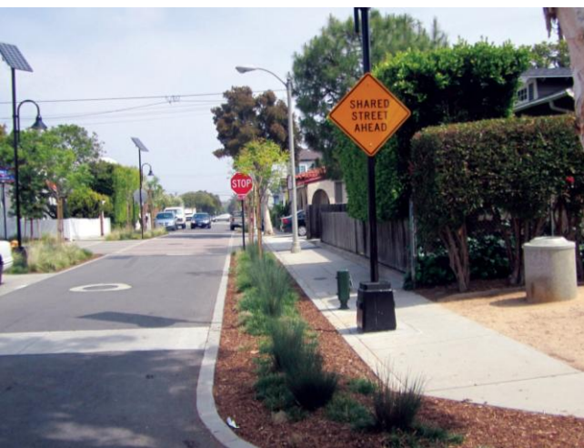
SANTA MONICA, CA Signage reinforces the transition to a shared street.
